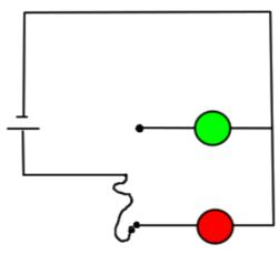
Extension Circuits can be further developed by having signals that allow a train to leave Platform 1 whilst the corresponding signals for Platform 2 are on red.
